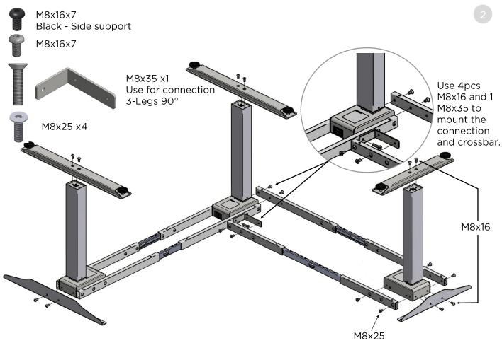
Note that there are two different fixing kits for mounting the table top. Only one is supplied depending on the chosen version of table top attachment.
